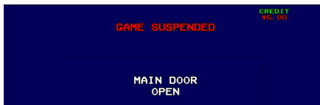
**Alarm + Key** = An Alarm will sound, and a Please Wait for the Attendant message will appear indicating which door is open. The Alarm will not Clear until the door is closed, and the Attendant has inserted and turned the Operator Menu Key.
