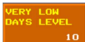
Displays the number of Days left before a Fill must be performed. Once the number of days falls below the set number an Alert Message will appear at the bottom left of the screen.
