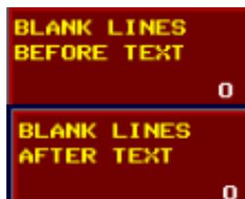
Tap to specify the number of blank lines preceding and following the text on tickets. These buttons can also be used to specify how much space is left between paper cuts and to center the text.
