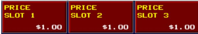
Tap each of the three **Price Slot** buttons to configure the amount of money added to the player's credit when a specific slot receives a pulse signal. Set this option at \$0.00 for a slot that is not in use.
