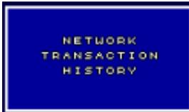
Tap to display a list of all the amounts that were transferred between the machine and the Network Controller when the machine is in Network System Mode
