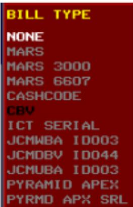
Tap to specify the brand and model of the bill acceptor connected to the gaming board. Selection is Highlighted in **White**.
