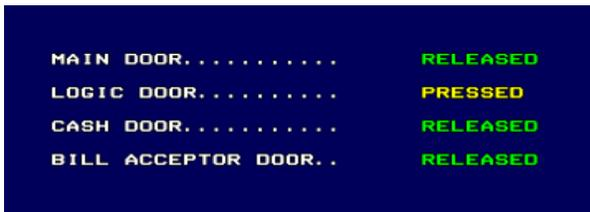
**Released** = Door is closed, or the Intrusion Switch is deactivated.
