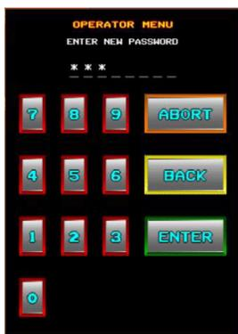
The BACK option appears only after the Operator has entered the second digit. The ENTER option appears only after the Operator has entered three digits. The code must contain from 3 to 8 digits.
