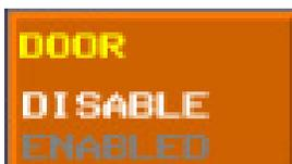
Tap to enable or to disable the Door option. When this option is enabled, doors close over the reels at the beginning of a round and open only to reveal the result.
