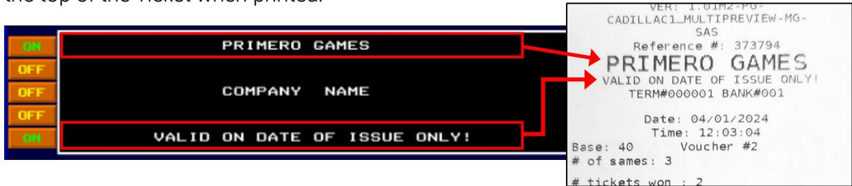
The Ticket Header allows for 5 lines of text. Each line can be turned on or off, if necessary, by Tapping the **ON** / **OFF** buttons to the left of each line.
