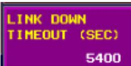
Tap to set the Link Down Timeout period. Default = 5400 sec or 90 minutes. Only available if the [Link Down Error](#) is Enabled.
