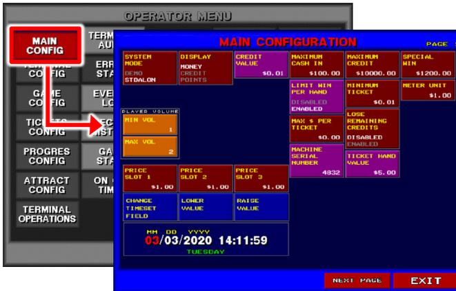
**Note:** Some options available in the Main Configuration Menus take effect only if the gaming machine contains a specific peripheral component, such as a hopper, a bill acceptor, or a tower light. Otherwise, the setting is ignored.
